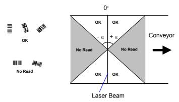
Figure 60 – Reading Zones with  $\alpha$  Max
