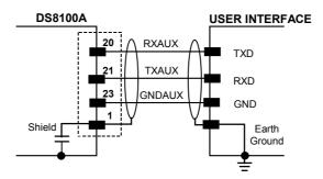
Figure 13 - RS232 Auxiliary Interface Connections
