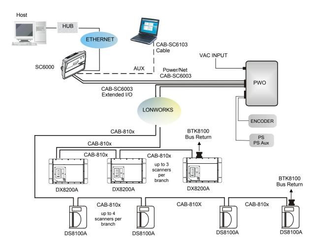
Figure 45 - Large Synchronized Network with DX8200A and DS8100A Scanners
