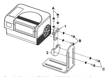
Figure 7 – Mounting the FBK-8100 and ST-163 Brackets on the Scanner
