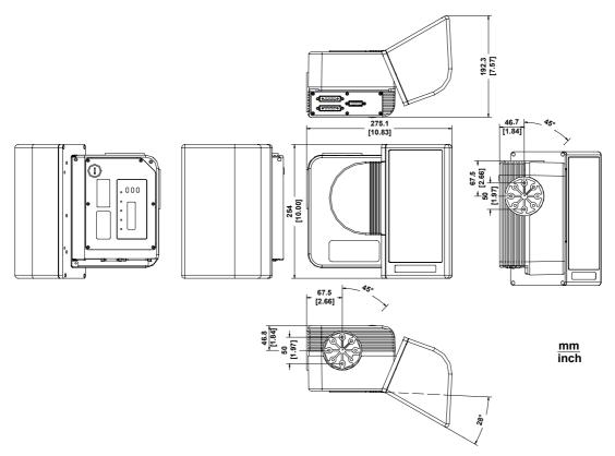
Figure 5 - DS8100A Oscillating Mirror Model Overall Dimensions
