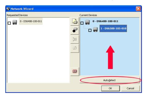
a. if the <u>slave scanners</u> have already been configured and <u>wired</u> to the network, click on the Autodetect button to start a polling procedure of the current network. All slave scanners found will be represented in the "Current Devices" area. Then, select the
