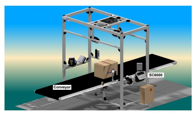
Figure 46 - Large Synchronized Network Reading Station
