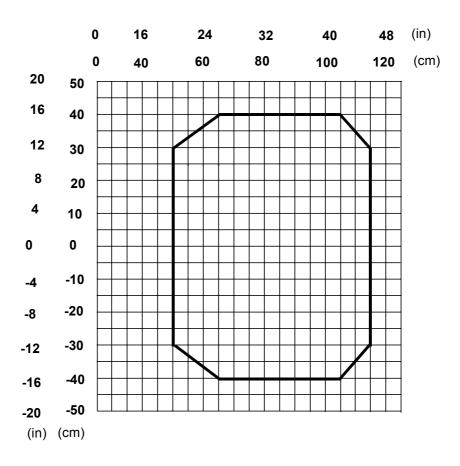
$\textbf{Note} \hbox{:}\ (0,0) \hbox{ is the center of the laser beam output window}.$
