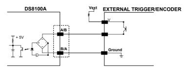
Figure 14 – PNP Command Input Connection using External Power
