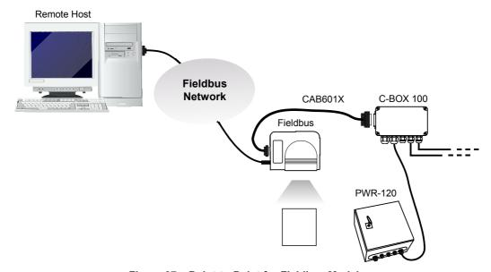
Figure 37 - Point-to-Point for Fieldbus Models
