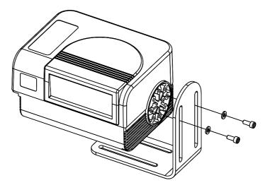
Figure 6 – Mounting the ST-163 Mounting Bracket
