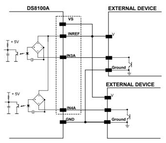
Figure 19 - IN3/IN4 NPN Input Command using Scanner Power
