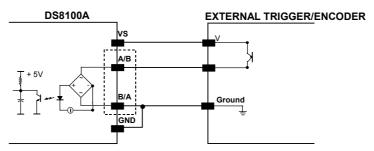
Figure 15 - PNP Command Input Connection using Scanner Power
