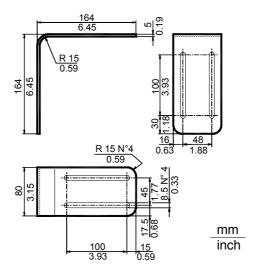
Figure 4– ST-163 Mounting Bracket Overall Dimensions
