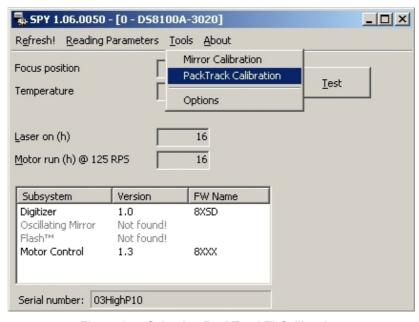
Figure 64 – Selecting PackTrack™ Calibration
