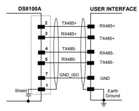
Figure 11 - RS485 Full-Duplex Interface Connections
