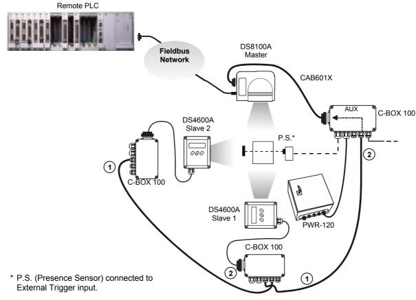
1 Main Serial Interface 2 Auxiliary Serial Interface
