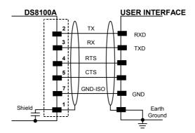
Figure 10 - RS232 Connections
