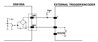
Figure 16 - NPN Command Input Connection using External Power
