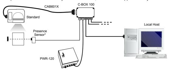
\* P.S. (Presence Sensor) connected to External Trigger input.
