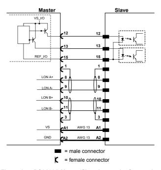
Figure 25 - DS8100A Master/Slave Lonworks Connection
