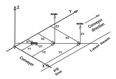
Figure 62 - DS Scanner PackTrack™ Reference System
