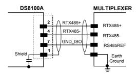
Figure 12 - RS485 Half-Duplex Interface Connections
