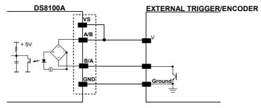
Figure 17 - NPN Command Input Connection using Scanner Power
