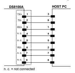
Figure 32 - Inverted Cable
