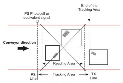
Figure 61 – PackTrack™ System Layout
