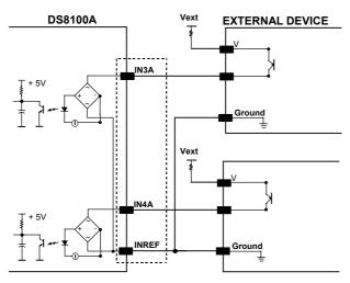
Figure 18 - IN3/IN4 PNP Input Command using External Power
