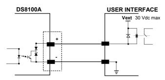
Figure 20 – Output 1 and Output 2 Interface
